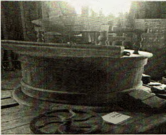
Messer Mayer ‘vat’ with a small door at the bottom set aside to show the opening for the Miller to take a test sample of ground meal.
